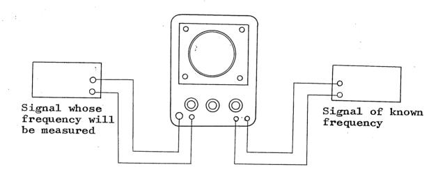
When the ratio of vertical frequency to horizontal frequency is integral in value, the figure on CRT stops showing one of the patterns illustrated below.
