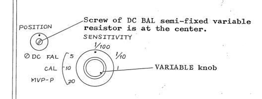
Adjustment of horizontal axis DC balance Conduct this adjustment 15 to 20 minutes after the 552F is energized.
