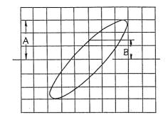
The intrinsic phase difference can be obtained as follows: Set the horizontal and vertical amplitudes of the loop figure to the scale as shown above, read values A and B, and calculate the phase difference angle by using the following formula:
